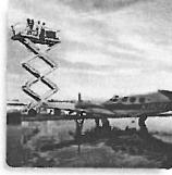
**SCISSORS LIFT** Photographers can use scissors lifts for overhead shots. The crossing beams of the lift form parallelograms that raise and lower the platform. For more about scissors lifts, see p. 300.
